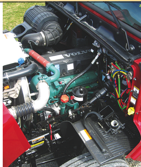
A D13 diesel, the only engine offered in the VHD, makes up to 485 horsepower and 1,650 lbs.-ft.
